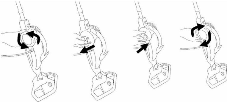
To replace the limescale filter, loosen the plastic cover on the „Handheld cleaner“, replace the filter and then close it again.
