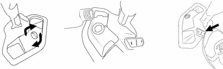
When cleaning a surface contaminated with grease, oil, etc., it is also possible to add a cleaning agent to the hot steam to increase the cleaning effect. Unscrew the „Cleaning solution tank cap“, pour the diluted cleaning solution into it and then close the tank again. Press the button to drain the cleaning solution to the „ON“ position.
