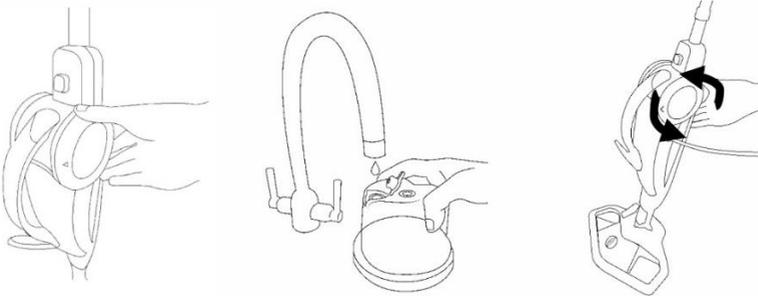
Remove the „Water tank“ from the main body by turning the side panel and pour water into it. Then carefully close the „Water tank“ and screw it back into the body of the steam mop.
