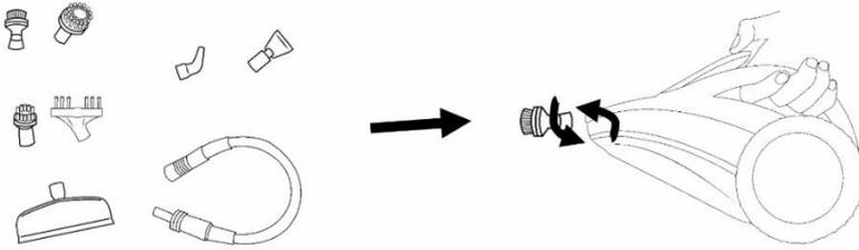
When using a flexi hose, connect it to the „Handheld cleaner“ until the button clicks. Choose a suitable cleaning attachment, place it on the „Handheld cleaner“ or flexi hose and turn it clockwise to firmly lock both parts.
