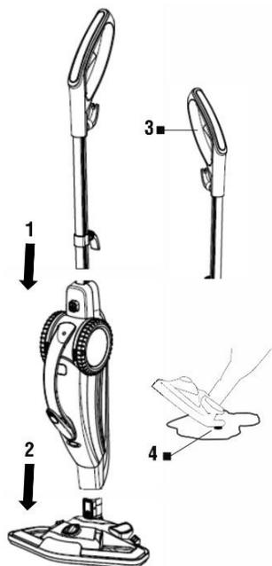
To fold the steam mop, insert the upper metal part (1) into the body of the appliance. Then also insert the lower mop head (2) into it.
