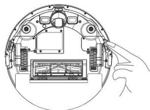
**Charging station connectors:** Disconnect the power supply and clean the contacts once a month with a soft, dry cloth.
