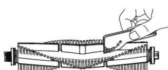
Remove the main central cleaning brush by pressing both handles on the brush cover. Use the cleaning tool to remove hair tangled in the main brush. Keep the center cleaning brush free of large amounts of hair, dust, cotton, etc. Check both side cleaning brushes together with the air intake hole, depending on the intensity of pollution, at least once a week, and remove tangled hair and other dirt from them.
