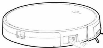
**Turn on:** set the switch button to the position **ON (1)**
